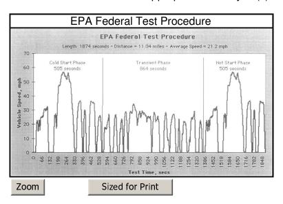
Manufacturers are required to validate monitors during the first 23 minutes (1372 seconds) of the Federal Test Procedure Drive Cycle.
