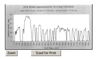
Completing the Drive Cycle successfully one (1) time should reset most drive cycle monitors to a "Ready" status. However, there are "two trip" monitors, which require that the drive cycle be successfully completed two (2) times, to achieve a "Ready" status. Furthermore, systems which use averaging, may require the drive cycle to be completed more than 2 times.
