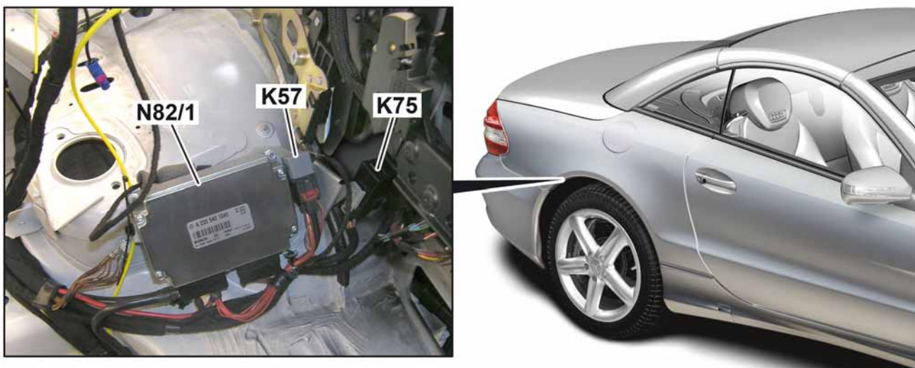
Location of vehicle power supply control unit and cutoff relay, shown on SL 500
