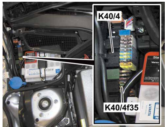
K40/4 Passenger-side fuse and relay module K40/4f35 Fuse 35 (20 A)
