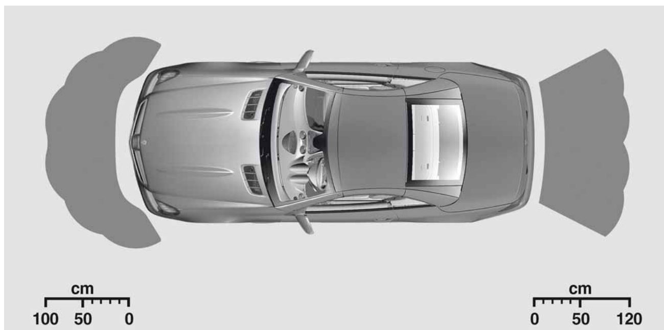
Monitoring range of PARKTRONIC distance sensors (schematic)
