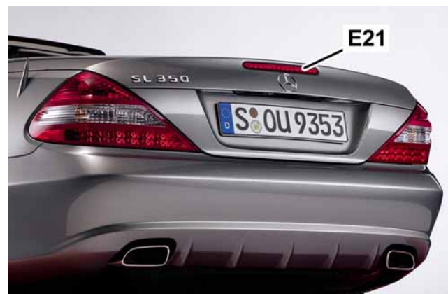
Center high-mounted brake lamp (E21) with LED technology
