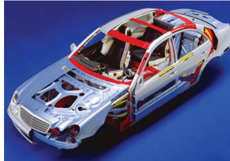
E-Class sedan body structure. HSLA steel is shown in red.
