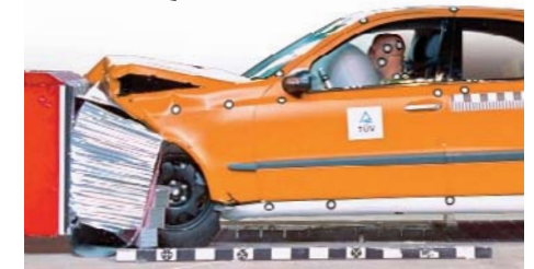
E-Class sedan in offset front impact crash test
