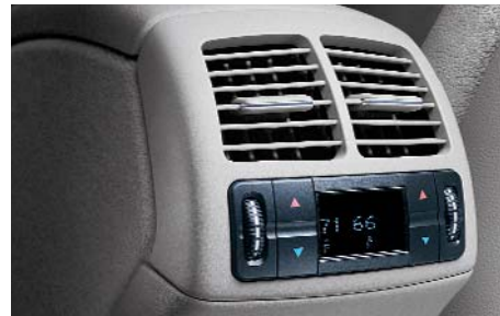
Rear-cabin control panel for 4-zone climate control
