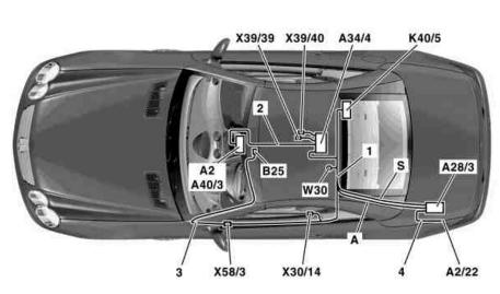
Wake-up signal/diagnosis distributor connector X30/14 X39/39 Handy connector
