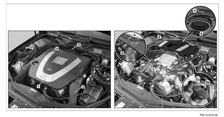
Front engine cover 1 Engine air intake duct 2
